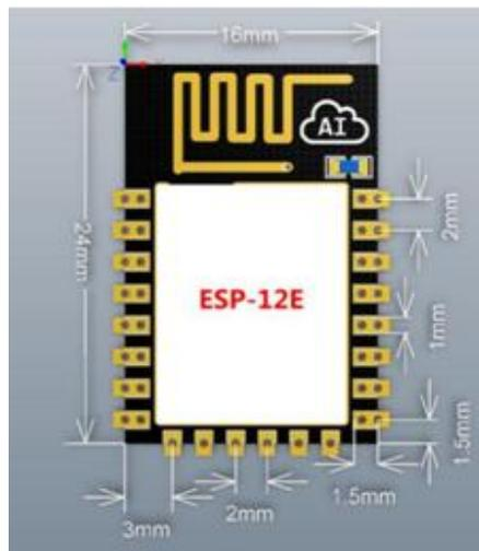
Figure 4 Top View of ESP-12E WiFi Module
