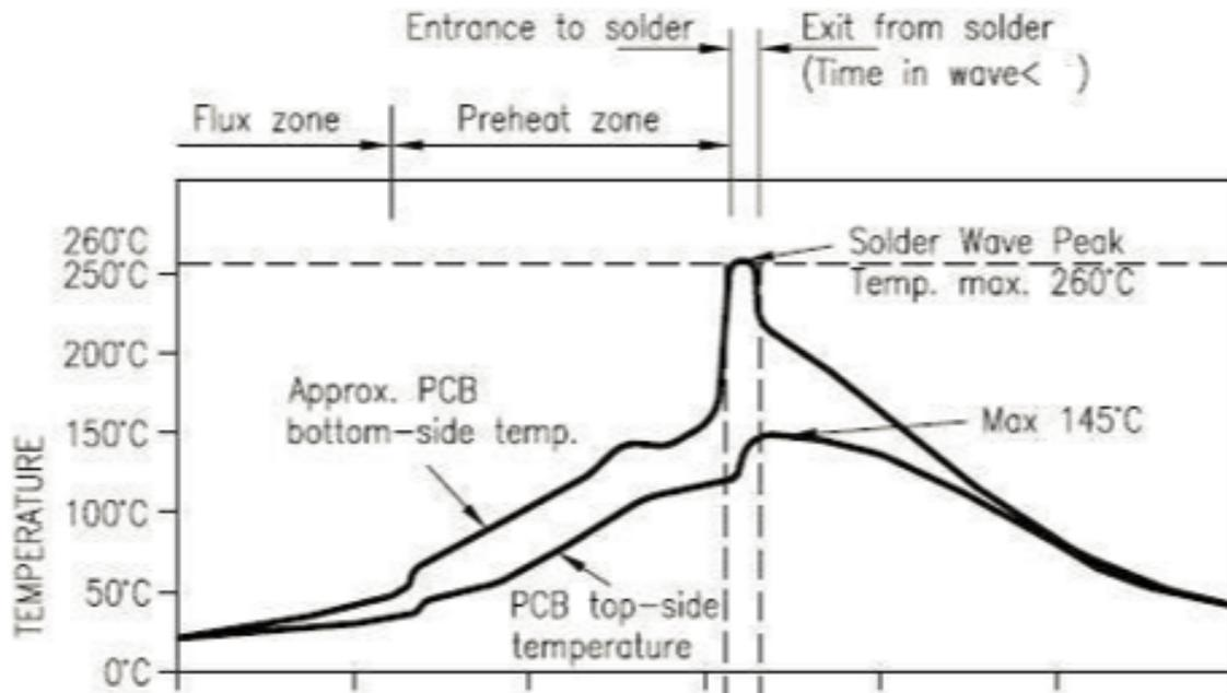
Suggestions on oven temperature curve of wave soldering
