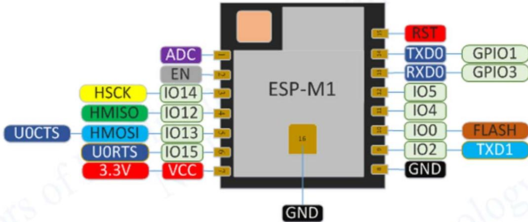
Fig. 2.1 ESP-M1 Definition for Pins
