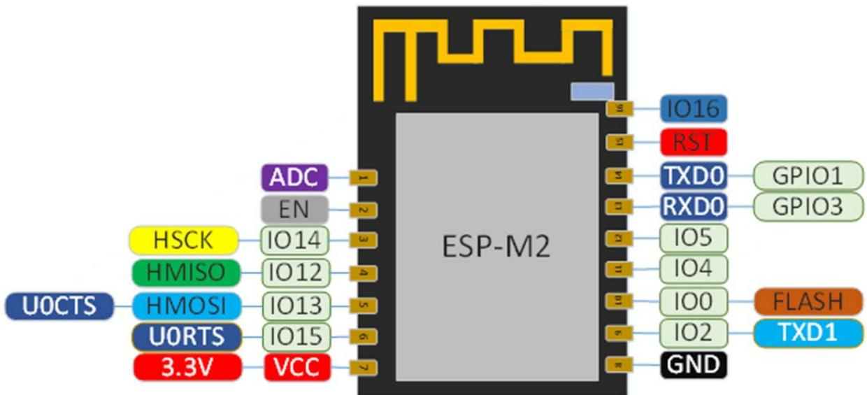
图 2.2 ESP-M2 Definition for Pins
