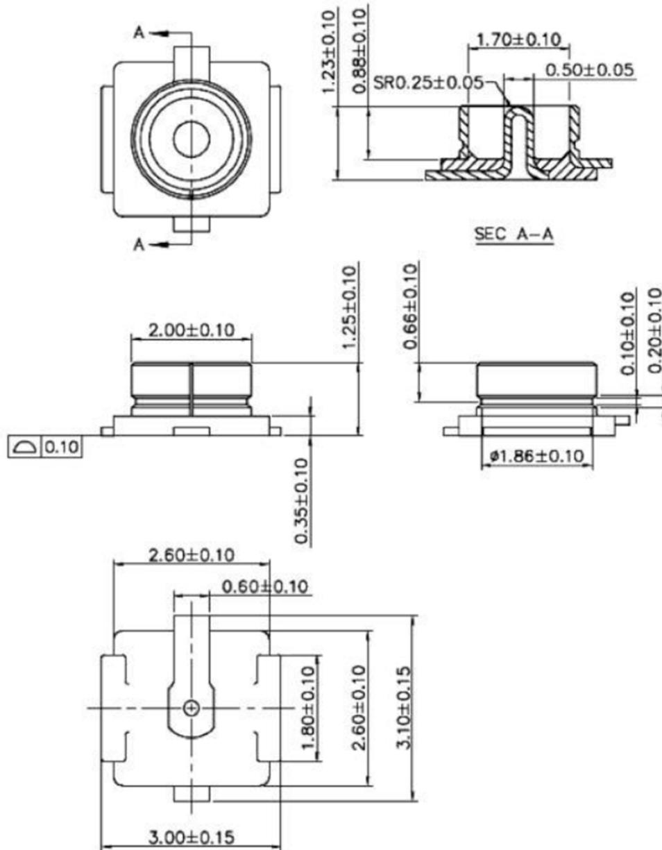
Fig. 9. 1 Connector for the external antenna
