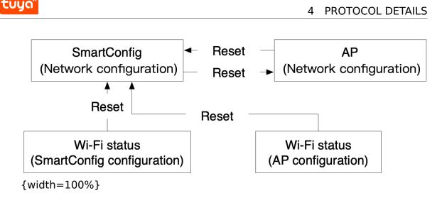
**Note**: When sending the reset command, please send it after the module initialization is completed. Otherwise, it may be invalid. For more information, see Wi-Fi Module Initialization Flow.
