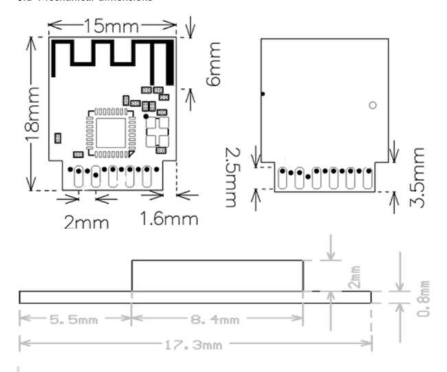
**Note**: The default dimensional tolerance is  $\pm 0.35$  mm. If a customer has other requirements, clearly specify them in the datasheet after communication.
