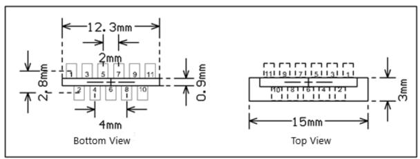
**Note**: The default dimensional tolerance is  $\pm 0.35$  mm. If a customer has other requirements, clearly specify them in the datasheet after communication.
